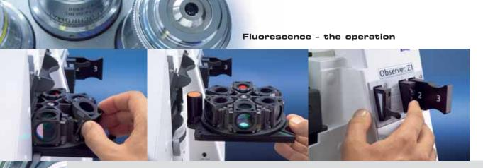
Reflector turret: in a matter of seconds, filter sets are now replaced without removing the reflector turret.
