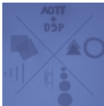
Fluorescent gel; rotated scanning fields and lines, and freely defined regions of interest show the performance capabilities of DSP and AOTF.
